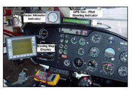
Cockpit displays for the pilot - HUMMINGBIRD EM system
