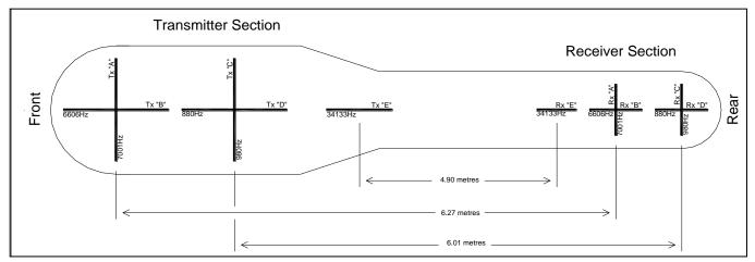
Layout and dimensions of the transmitter and receiver coils in the HUMMINGBIRD EM sensor
